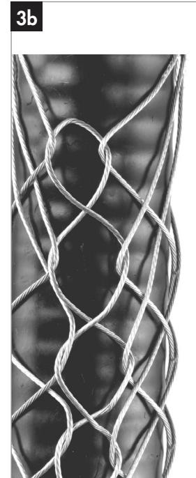
**4** Continue lacing so that the seam is straight and the lace is pulled so that the space between both sides of the seam is no greater than the spaces of the mesh next to the loop. See Figure 4. **Do not skip any loop pairs of the grip when lacing;** this will weaken the hoisting grip. The grip can be compressed from bottom to top to simplify lacing.
