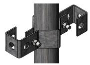
PIM-Guard® Round Member Cable Support Bracket 6 ports for stackable hangers (up to 3 per port). Install with torque wrench set at 5 to 7 ft-lb to meet carrier PIM requirements. For patents, see www.cs-pat.com
