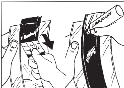
5.4 Remove the protective paper from the inside of the sealing strip. Lubricate abundantly.
