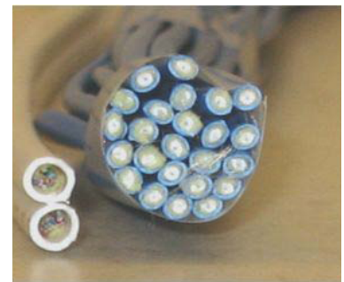
Dual 12-Fiber 3.0 mm Microcables Compared with 24-Fiber Breakout Cable
