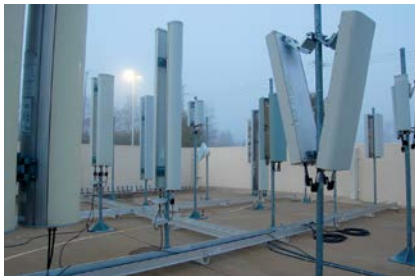
12.8: UV and weathering test of base station antenna assemblies
