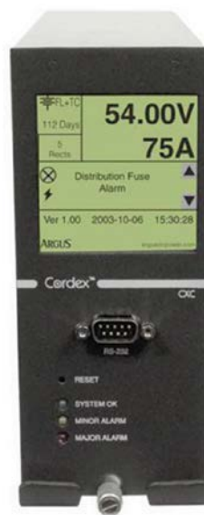
11.12: A system controller interface displaying voltage, amperage and alerts
