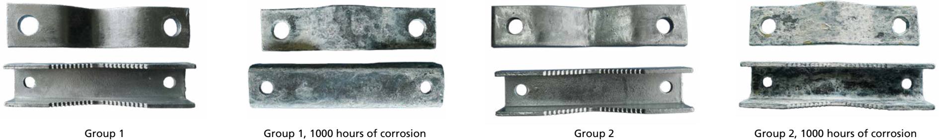
12.7: Weathering and corrosion test of silver-plated steel products
