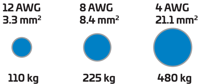
Figure 7: Approximate weight of 60-meter power/fiber cables for 12 RRUs
