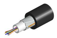
Fiber Indoor/Outdoor Drop Cable, LazrSPEED®, Low Smoke Zero Halogen Single Jacket All-Dielectric Arid-Core, 12 fiber, Gel-filled, Multimode OM3, Feet jacket marking, Black jacket color, Dca flame rating
