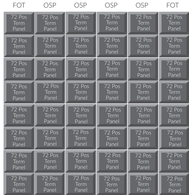
Figure 16. ODF cross-connect configuration with 2:1 OSP:FOT ratio
