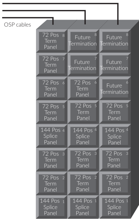
ODF with splicing and terminations located in central office. (3) frames, total capacity: 1080 terminations.
