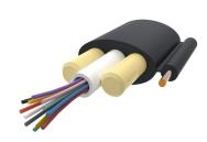
Fiber Hybrid drop cable, LightScope ZWP® Fiber + Tone Wire Outdoor, 2 fiber Arid Core construction, central loose tube, Gel-filled, Singlemode G. 652.D and G.657.A1, Feet jacket marking, Black jacket color
