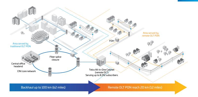
As telco networks expand farther from the central office, more active and passive distribution cabinets are needed at the edge of the OSP network. These large cabinets can be visibly obtrusive. While some can be integrated into larger utility structures such as cell tower base stations or power substations, most must be deployed as standalone units, subject to local land use requirements and approval processes. For operators needing to accelerate the turnup of new customers, any delay is costly.
