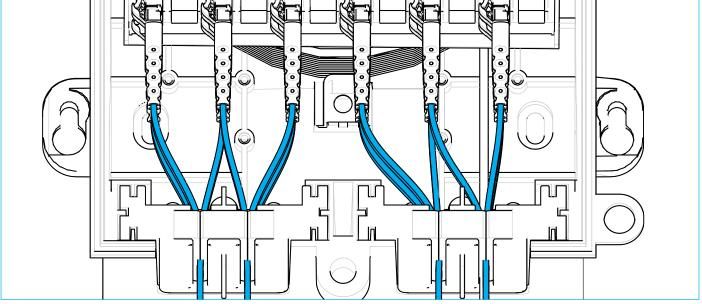
10.5 Route the patch cords through the drop cable foam seal as shown above.
