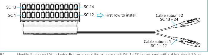
9.1 Identify the correct SC adapter. Bottom row of the adapter pack (SC 1 - 12) correspond with cable subunit 1 (see brady label on connector at the cable end). Top row of the adapter pack (SC 13 - 24) correspond with cable subunit 2. **Important:** It is important to install first bottom row (SC 1 - 12) adapters.
