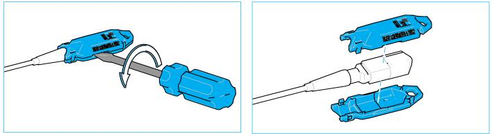
8.6 For **MPO connectors**: At the termination point, remove the pulling eye and connect the cable connector to the termination point adapter.
