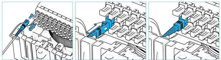
Remove dust cap from selected SC adapter and connector of the patch cord and clean per local practise. 9.2 Note: The adapter pack cover is removable for connector cleaning. **Note:** Remove ferrule dust cap from one of the patch cord connectors and then clean connector as specified in the Optical Fiber Connector Wet and Dry Cleaning Instructions (ADCP-90-159) or by locally approved procedures.
