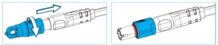
8.7 For **HMFOC connectors**: Remove the dustcap and connect the cable connector to the termination point adapter. **Note:** the connectors are labeled. Make sure to select the correct connect to the designated adapter port (see section 9.1).
