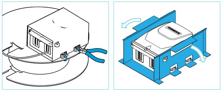
6.1 If applicable, remove the BUDI-R from the external spool by cutting the cable ties. **Note**: Unwind the loop of cable within the lead loop holder.
