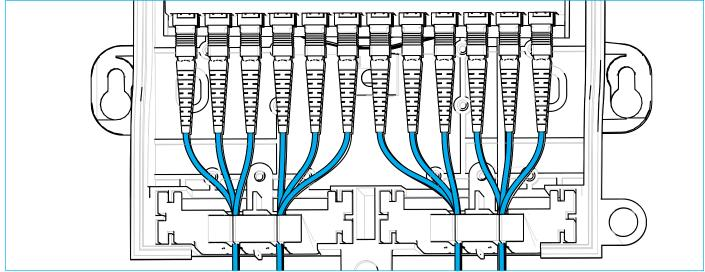
Route the patch cords through the drop cable foam seal. The first 3 cords are routed to the first slot in the foam 9.5 seal, second 3 cords to the next slot and so on.
