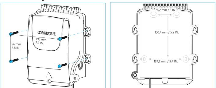
7.1 Use the BUDI-R as a template to mark the mounting screw locations on the wall selected for the installation location. (Inside or mounting ears at the outside the box).
