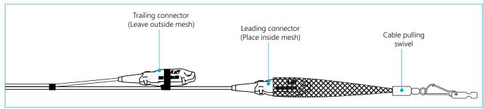
5.1.1 Insert the leading connector pulling eye (installed in the factory) into the pulling swivel mesh.
