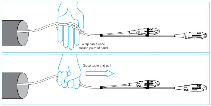
5.3.2 At the conduit exit location, remove the tape, mesh, and pulling swivel from the leading connector pulling eye(s), and use the hand-wrap method shown to pull the cable to the point where the cable will be terminated.
