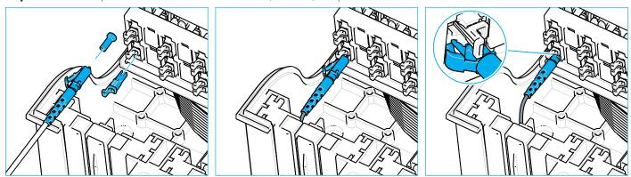
10.2 Remove dust cap from selected LC adapter and connector of the patch cord and clean per local practice. **Note:** The adapter pack cover is removable for connector cleaning. **Note:** Remove ferrule dust cap from one of the patch cord connectors and then clean connector as specified in the Optical
