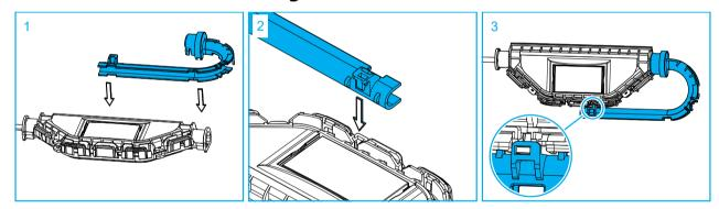
1 Install the fiber cable guide as shown in the pictures above until it snaps onto the SRC10 closure.
