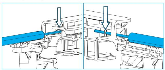
If a rigid central strength member is present, cut it back to 3 + 0/-0.5 cm / 1.18 + 0/-0.2 Inches. To prevent damage due to strength member pistoning effects, the strength member should be installed as shown in the images above.
