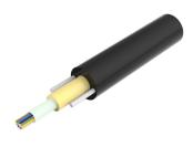
Optical Fiber OSP Drop cable, HDPE jacket, ST buffer, Singlemode, G.657. A2, 12 fiber, meter marked, black jacket color. Box Packaged in 500m lengths.
