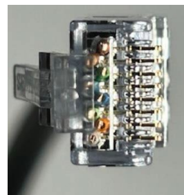
Copper ends of conductors fully inserted
