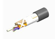
Fiber indoor/outdoor cable, TeraSPEED®, Single Jacket All-Dielectric, Plenum Rated, Multimode/Singlemode, 48 fiber, Gel-Free, Stranded Loose Tube, PVDF jacket, Black jacket color, Feet cable marking
