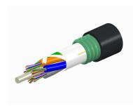
Fiber OSP cable, TeraSPEED® Single Jacket/Single Armor, Gel-Free, Stranded Loose Tube, 72 fibers, Composite OM4 and G.652.D and G.657. Al, Feet jacket marking, Black jacket color
