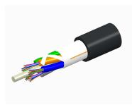
Fiber OSP cable, TeraSPEED® Single Jacket All-Dielectric, 240 fiber, Gel-Free, Stranded Loose Tube, Singlemode G.652.D and G.657.Al, Feet jacket marking, Black jacket color
