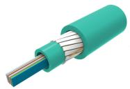
Fiber Indoor Cable, Plenum All-Dielectric Central Tube Ribbon, 72-fiber, Multimode OM4 bend insensitive, Feet jacket marking, Aqua jacket color
