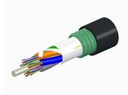
Fiber indoor/outdoor cable, TeraSPEED®, Single Jacket/Single Armor, Low Smoke Zero Halogen (LSZH), 96 fiber, Singlemode G.657.A2, Gel Filled , Stranded Loose Tube, Black jacket color, Meters jacket marking, Cca flame rating
