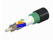
Fiber indoor/outdoor cable, TeraSPEED®, Single Jacket/Single Armor, Low Smoke Zero Halogen (LSZH), 144 fiber, Singlemode G.657.A2, Gel Filled , Stranded Loose Tube, Black jacket color, Meters jacket marking, Cca flame rating
