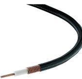
FSJ4RK-50B, HELIAX® Superflexible Foam Coaxial Cable, corrugated copper, 1/2 in, black non-halogenated, fire retardant polyolefin jacket B2ca-sla-d1-a1 (CPR testing is conducted annually please reference the website for latest classification)
