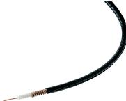
Heat Treated FSJ1RK-50B, HELIAX® Superflexible Foam Coaxial Cable, corrugated copper, 1/4 in, black non-halogenated, fire retardant polyolefin jacket
