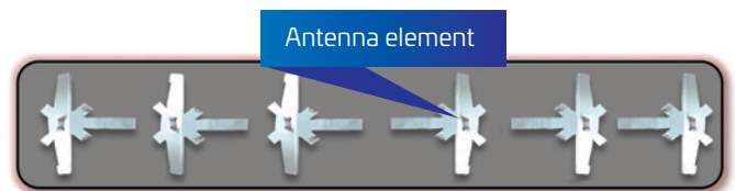
Figure 3, Base station panel antenna
