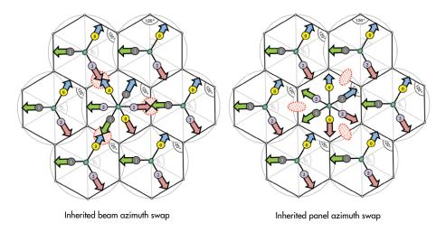
The first arrangement (inherited beam azimuth) is thus recommended, after necessary **tilts adjustments**, to overcome the direct shooting bores.
