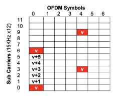
**V-shift** is used to shift the RS frequency allocations between neighboring sectors, reducing interference.
