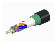
Fiber OSP cable, LightScope ZWP® Single Jacket/Single Armor, 240 fiber, Gel-Free, Stranded Loose Tube, Singlemode G.652.D and G.657.Al, Feet jacket marking, Black jacket color
