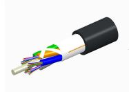
Fiber OSP cable, LightScope ZWP® Single Jacket All-Dielectric, 184 fiber, Gel-Free, Stranded Loose Tube, Singlemode G.652.D and G.657.A1, Feet jacket marking, Black jacket color
