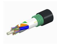
Fiber indoor/outdoor cable, LightSCOPE® Indoor/Outdoor, Single Jacket /Single Armor, Low Smoke Zero Halogen (LSZH), Singlemode G.652.D and G.657.A1, 144 fiber, Gel Filled, Stranded Loose Tube, Feet jacket marking, Black jacket color, Cca flame rating
