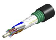
Fiber OSP cable, LightScope ZWP® Mini Single Jacket/Single Armor, 144 fiber, Gel-Filled, Stranded Loose Tube, Singlemode G.652.D and G.657.A1, Meters jacket marking, Black jacket color
