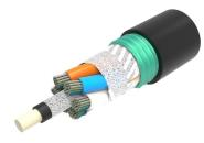
Fiber OSP cable, Outdoor Steel Armored, Gel-Free, Stranded Loose Tube Rollable Ribbon, 1152 fiber, Singlemode G.652.D and G.657.A1, Feet jacket marking, Black jacket color
