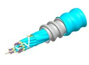
Fiber indoor cable, LazrSPEED® Riser/LSZH rated, MPO Trunk, interlocking aluminum armored, Multimode OM4, 12 fiber, Gel-free, Feet jacket marking, Aqua jacket color, B2ca flame rating
