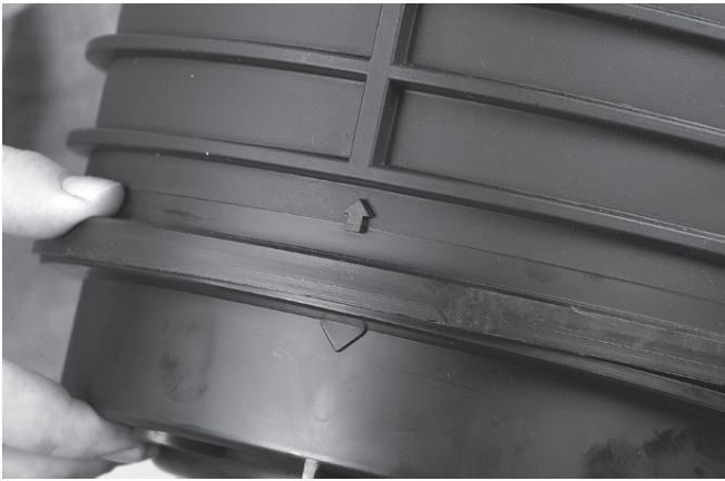
9.6 Slide the dome onto the base. Make sure that the arrows match. Use the clamp to seal dome and base.
