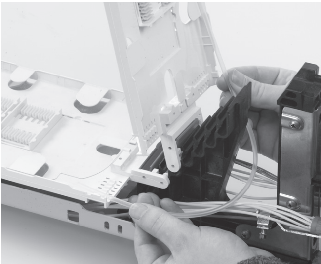
6.2.5 Inter tray jumping. Route the transportation tube from the bottom tray, behind the tower, over the already installed loose tubes to the allocated tray.
