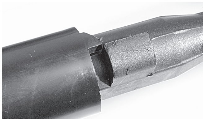
9.4 Tighten the trigger until it butts. If necessary, use wrench to tighten the trigger.
