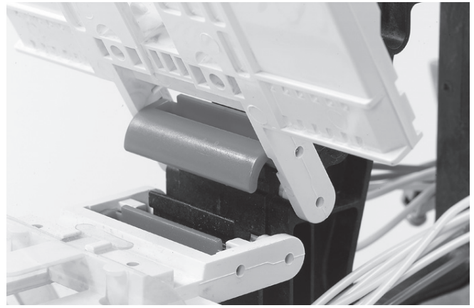
6.2.6 The tray can be blocked with the tray wedge. Turn the wedge to the shown position.
