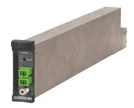
The receiver utilizes Avalanche Photo Diode (APD) technology, enabling very high receiver sensitivity to extend link reach. The receiver supports an optical input range of to -23 to -10 dBm.
