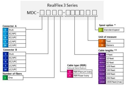
\*Drops are automatically coiled 0-350 ft. Lengths 351+ are automatically spooled. Connector A deploys first. Add option J if spool is required for lengths 350ft or less. \*\*Cable length shown as an example; additional cable lengths available upon request up to 1500 ft
