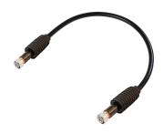
HELIAX® 1/2" SureFlex® Fire retardant Jumper with interface types 4.3-10 Male and 4.3-10 Male with HELIAX® SureGuard weatherproofing, with black non-halogenated fire retardant polyolefin jacket B2ca-Sla-dl-al
