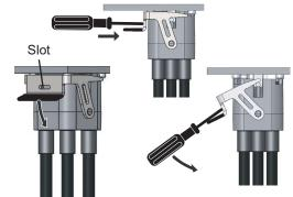
Grasp M-LOC connector housing, hold bent flange portion of latch back toward cable strain relief, pull the connector away from device. A slight back and forth motion on the housing helps to release the port connectors.
