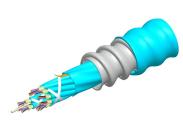
Fiber indoor cable, LazrSPEED® Riser/LSZH rated, MPO Trunk, interlocking aluminum armored, Multimode OM4, 48 fiber multi-unit with 12 fiber subunits, Gel-free, Feet jacket marking, Aqua jacket color
