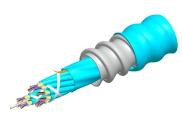
Fiber indoor cable, LazrSPEED® Riser/LSZH rated, MPO Trunk, interlocking aluminum armored, Multimode OM4, 48 fiber multi-unit with 12 fiber subunits, Gel-free, Feet jacket marking, Agua jacket color
