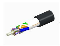
Fiber indoor/outdoor cable, LightSCOPE ZWP® Single Jacket All-Dielectric, 12 fiber, LSZH, Gel-Free, Stranded Loose Tube, Singlemode G. 652.D and G.657.Al, Meters jacket marking, Black jacket color, Eca flame rating
