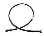
HELIAX® 1/2" Superflexible Fire retardant SureFlex® Jumper with interface types N Male and N Female, 0.5 m, with black non-halogenated fire retardant polyolefin jacket
