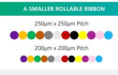
Partially bonded individual 200 $\mu m$  fibers  ${\sim}25\%$  smaller cable OD than 250 $\mu m$  rollable ribbon constructions
