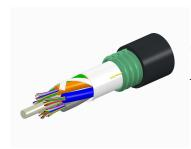
Fiber OSP cable, LightScope ZWP® Single Jacket/Single Armor, 96 fiber, Gel-Free, Stranded Loose Tube, Singlemode G.652.D and G.657.A1, Feet jacket marking, Black jacket color
