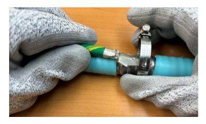
2. Using ¼" socket or nut driver, tight hose clamp, torque at 14-16 in-lbs.
