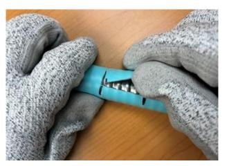
3. Verify that ground terminal makes good contact with non-jacketed armored cable.
