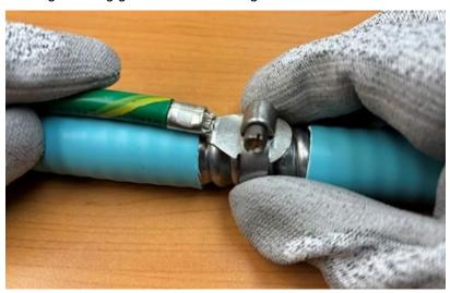
2. Using ¼" socket or nut driver, tight hose clamp, torque at 14-16 in-lbs.
