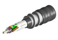
Fiber indoor/outdoor cable, TeraSPEED®, Plenum Rated, Singlemode G. 652.D and G.657.A1, Gel-Free, 96 fiber, Stranded Loose Tube with Aluminum Interlocking Armor containing a Plenum Rated Outer Jacket, Black jacket color, Feet cable marking
