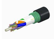
Fiber OSP cable, TeraSPEED® Single Jacket/Single Armor, 156 fiber, Gel-Free, Stranded Loose Tube, Singlemode G.652.D and G.657.A1, Feet jacket marking, Black jacket color
