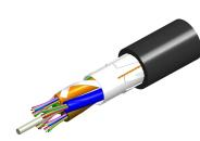
Fiber OSP cable, LazrSPEED®, Light Duty, Single Jacket, All-Dielectric, 36 fiber, Gel-Free, Stranded Loose Tube, Multimode OM3, Feet jacket marking, Black jacket color
