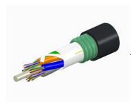
Fiber OSP cable, TeraSPEED® Single Jacket/Single Armor, 96 fiber, Gel-Free, Stranded Loose Tube, Singlemode G.652.D and G.657.Al, Meters jacket marking, Black jacket color
