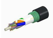
Fiber OSP cable, TeraSPEED® Single Jacket/Single Armor, 144 fiber, Gel-Free, Stranded Loose Tube, Singlemode G.652.D and G.657.A1, Meters jacket marking, Black jacket color
