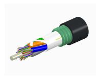
Fiber OSP cable, TeraSPEED® Single Jacket/Single Armor, 120 fiber, Gel-Free, Stranded Loose Tube, Singlemode G.652.D and G.657.A1, Feet jacket marking, Black jacket color
