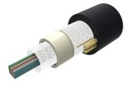
Fiber OSP Cable, Non-Armored, All-Dielectric, Arid-Core, Dry Central Tube Ribbon, 36 fibers, Singlemode G.652.D and G.657.A1, Gel-free, Feet jacket marking, Black jacket color
